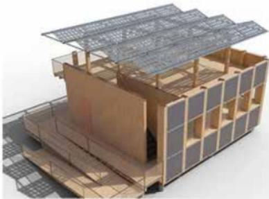
Like the Café Ada extension, the unit is divided into layers. The service layer includes the kitchen, the bathroom, the entrance area and the building utilities.
