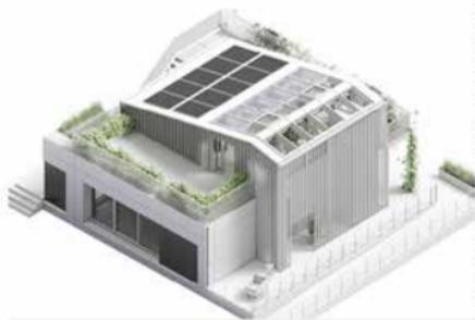
The HDU consists of three wood modules on the ground floor that closely resembles the original design of the rooftop extension.
