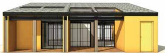
The house demonstration unit (HDU) is selected at the roof top position where sun room is located. The approach the solar heat gain from clean energy of sunlight is applied high-performance glazing. Together with recycling wall and floor material, we expected the heat is collected into the materials for releasing mean radiant temperature at night with naturally ways.
