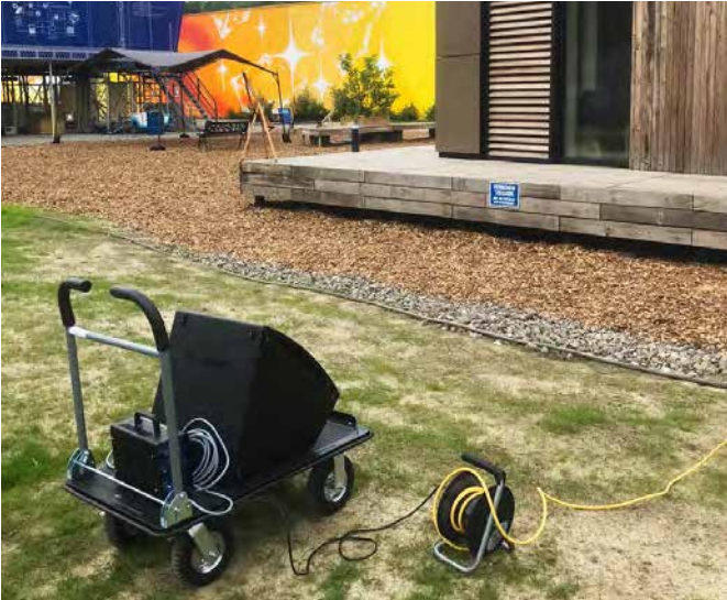
Based on the targeted use of a sound source outdoors, the resulting sound level was measured indoors. © SDE 21/22
